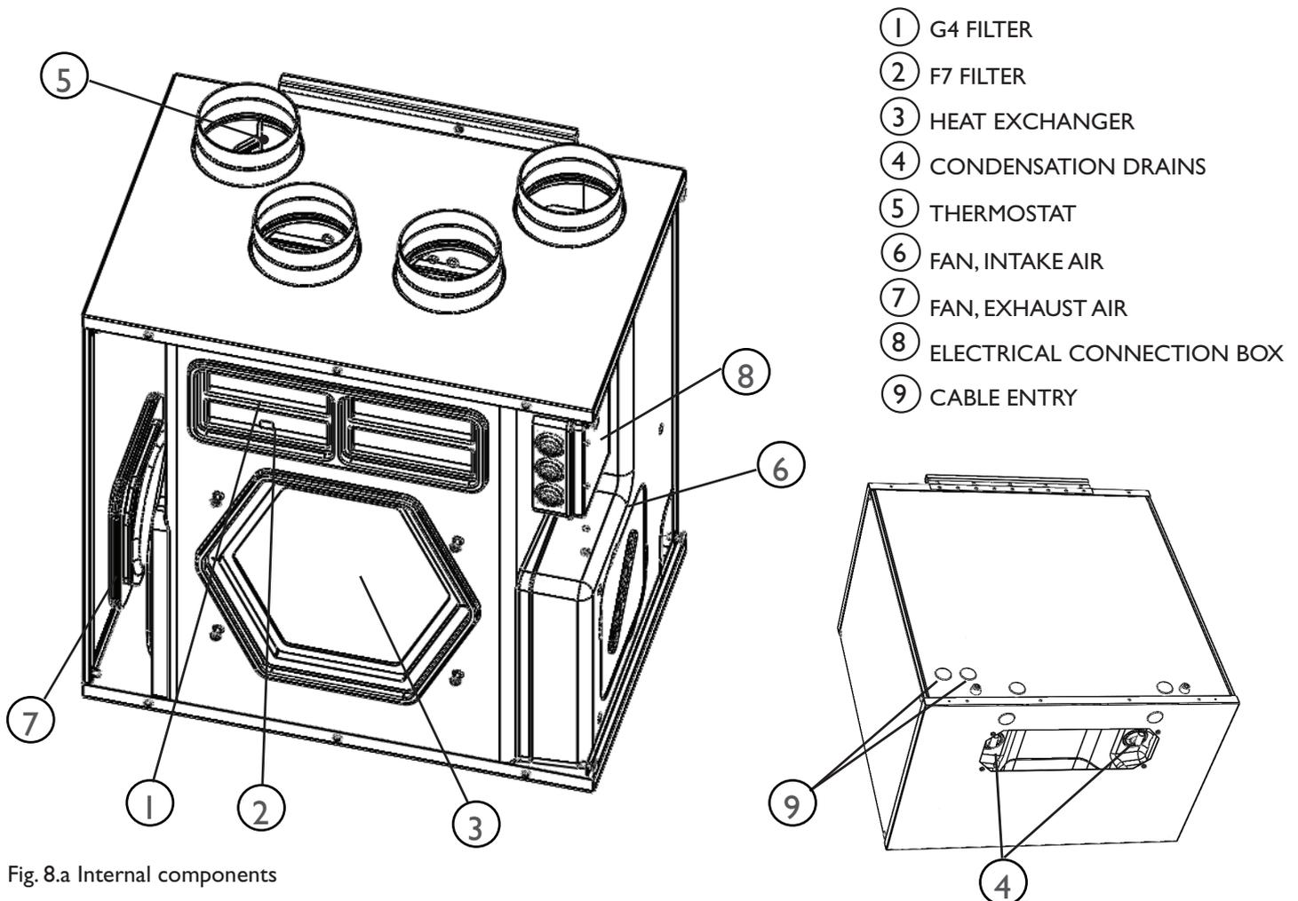
Fig. 8.a Internal components
