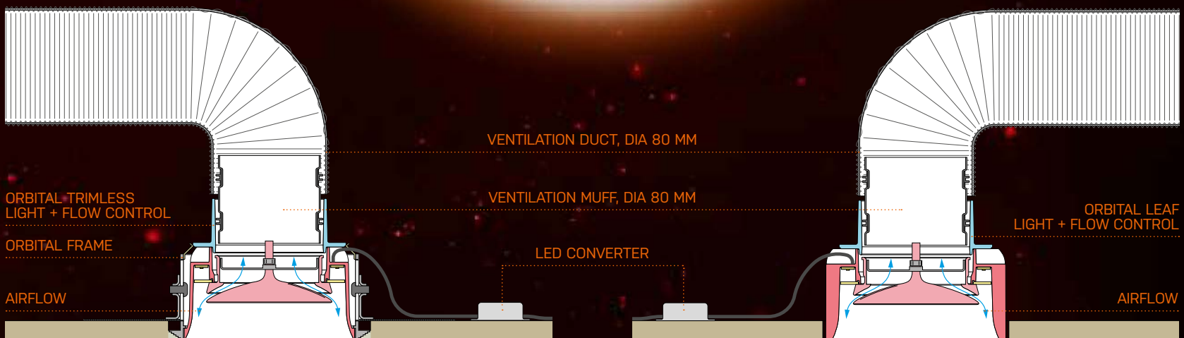
ORBITAL TRIMLESS LIGHT + FLOW CONTROL (ventilation + adjuster)
